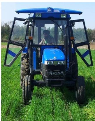
Fig. 4: View of Installed N-sensor on the Tractor Roof in the Field
