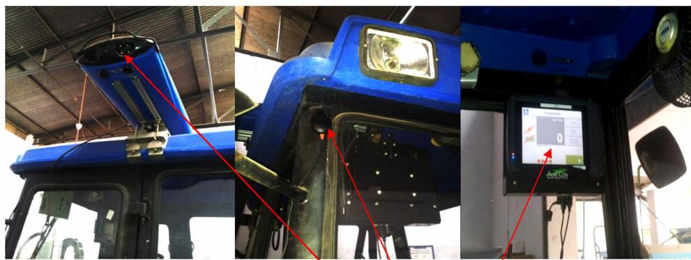
Fig. 2: View of N-sensor Viewing Angle, DGPS and Computer Screen
