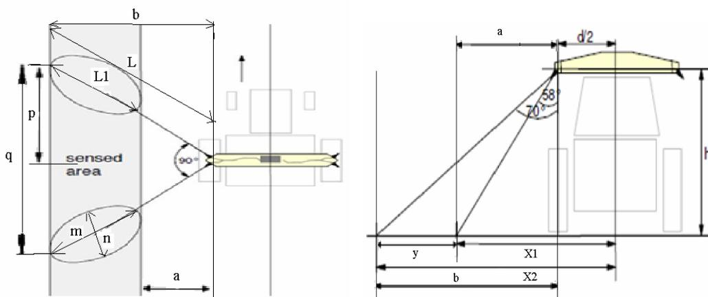
Fig. 3: Top and Front View of Geometry of N-Sensor (all dimensions are in meter)
